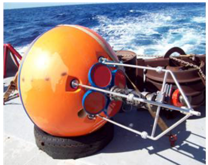
Fig. 1. The mooring equipped with Teledyne RDI ADCP (Workhorse Longranger 75 kHz).
