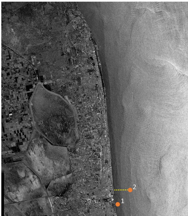
Fig. 2. ADCP mooring locations superimposed on an ERS-2 satellite SAR image. The SAR image was taken on 19 November 2009; wind speed was 4.9 \text{ m s}^{-1} and wind direction 348^\circ (meteorological convention). Corner points of the SAR image are 27.088^\circ\text{N} , 80.482^\circ\text{W} ; 26.902^\circ\text{N} , 79.486^\circ\text{W} ; 26.097^\circ\text{N} , 80.709^\circ\text{W} ; 25.912^\circ\text{N} , 79.723^\circ\text{W} . Label 1 is the bottom ADCP mooring, at an 11-m isobath on the Dania Beach shelf ( 26.073^\circ\text{N} , 80.101^\circ\text{W} ), and Label 2 is the bottom ADCP mooring 8 nautical miles (14.8 km) offshore at a 244-m isobath ( 26.191^\circ\text{N} , 79.974^\circ\text{W} ). The dotted line represents the R/V F.G. Walton Smith transect repeated approximately every two months (see Figs. 7–8).
